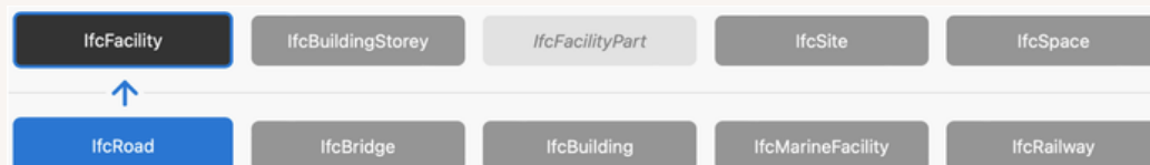
Slika 20: Shema razredov IFC 4.3.1.0 (IFC4x3_ADD1) za ceto, vir: https://ifc43-docs.standards.buildingsmart.org/IFC/RELEASE/IFC4x3/HTML/lexical/IfcRoad.htm
