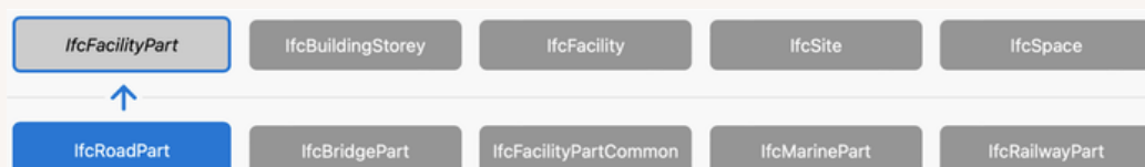
Slika 21: Shema razredov IFC 4.3.1.0 (IFC4x3_ADD1) za del ceste, vir: http://ifc43-docs.standards.buildingsmart.org/IFC/RELEASE/IFC4x3/HTML/lexical/IfcRoad.htm
